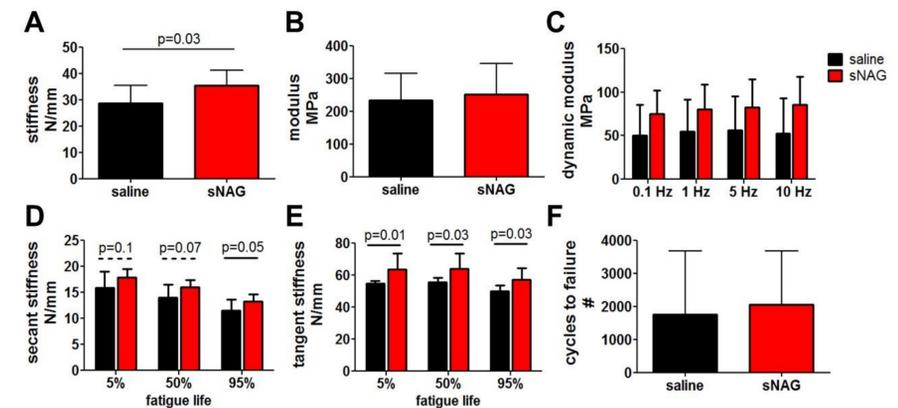
**Figure 2. Mechanical Properties.** Three weeks after injury, sNAG treated tendons had (A) increased stiffness, (B) no change in modulus, (C) increased dynamic modulus across testing frequencies, (D) increased secant stiffness, and (E) increased tangent stiffness. There were no changes in (F) cycles to failure between groups. Data shown as mean±SD.
