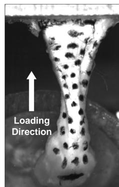
**Figure 1. Achilles mechanical testing.** Calcaneus-foot complex in PMMA with stain dots for optical strain tracking.
